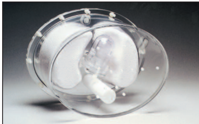
Lung-Spine Phantom shown with Cardiac Insert in place and Elliptical Cylinder
