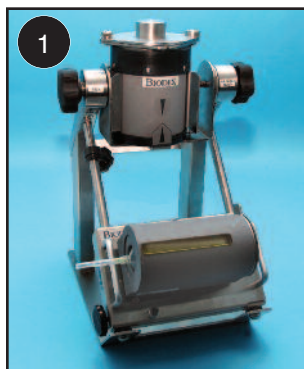
Syringe shield mounts to the stand on a stainless steel rotating platform; syringe is placed in shield. Note vial shield in upright position.
