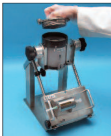
Vial shield shipping cover is replaced with the drawing shield cover.
