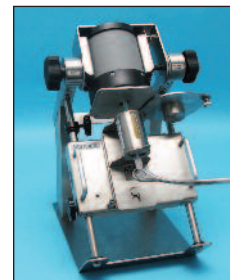
Syringe shield slides upward, allowing the syringe to puncture the vial septum. Dose is drawn.
