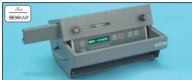
Lead glass window offers 5.6 density with clear visibility of syringe.
