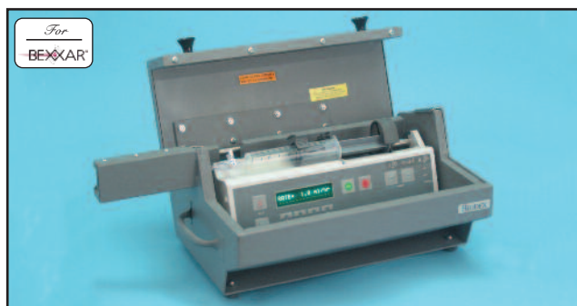
The shield cover, when open, acts as a protective barrier; stand behind the pump to insert the syringe.
