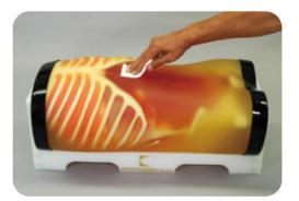
Wipe the remaining gel completely by wet cloth. If remaining gel gets dried up on the body, it may cause scratches and tears on the phantom material.
