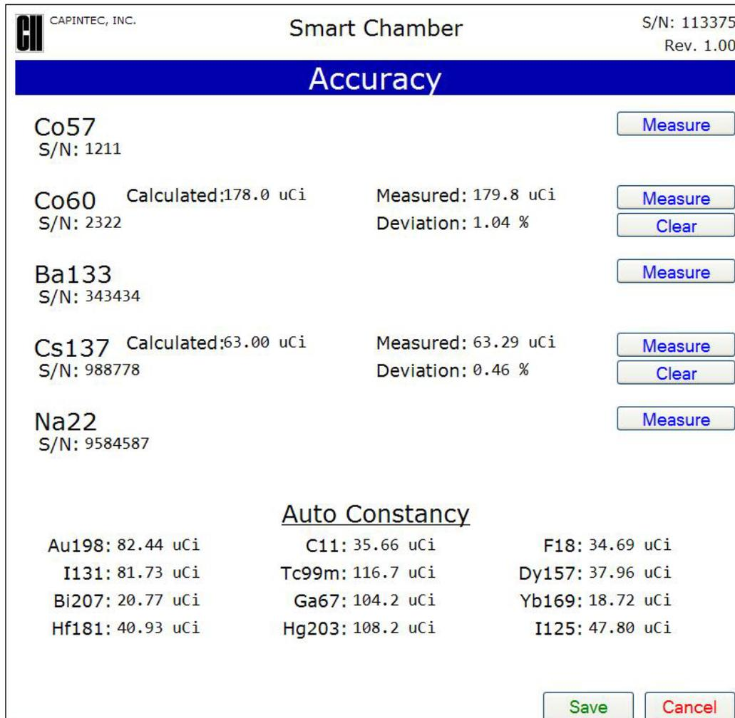
Figure 8-7 Accuracy/Constancy Results Screen
