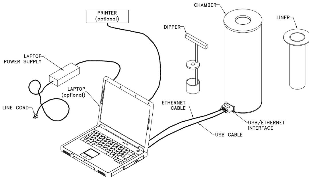
Figure 4-2 Configuration 2 with Optional Accessories
