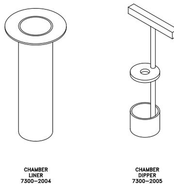
Figure 4-6 Liner and Dipper
