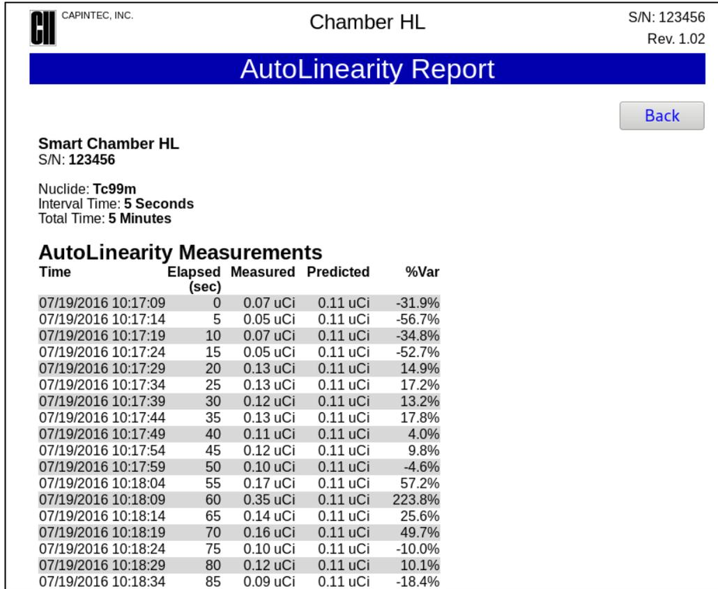
Figure 8-14 Completed AutoLinearity Test Report
