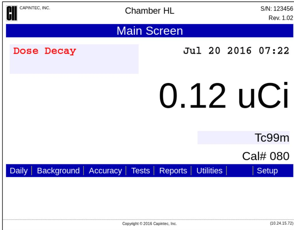
Figure 4-5 Main/Measurement Screen
