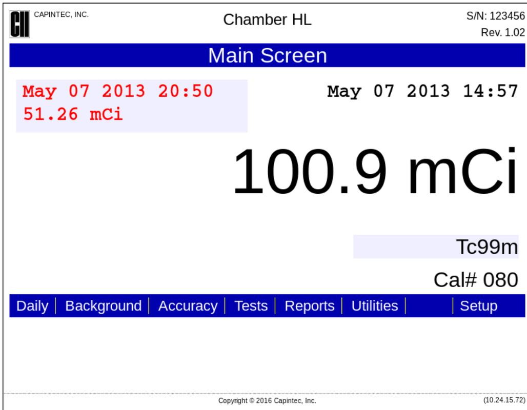
Figure 10-4 Main/Measurement Screen with Dose Decay
