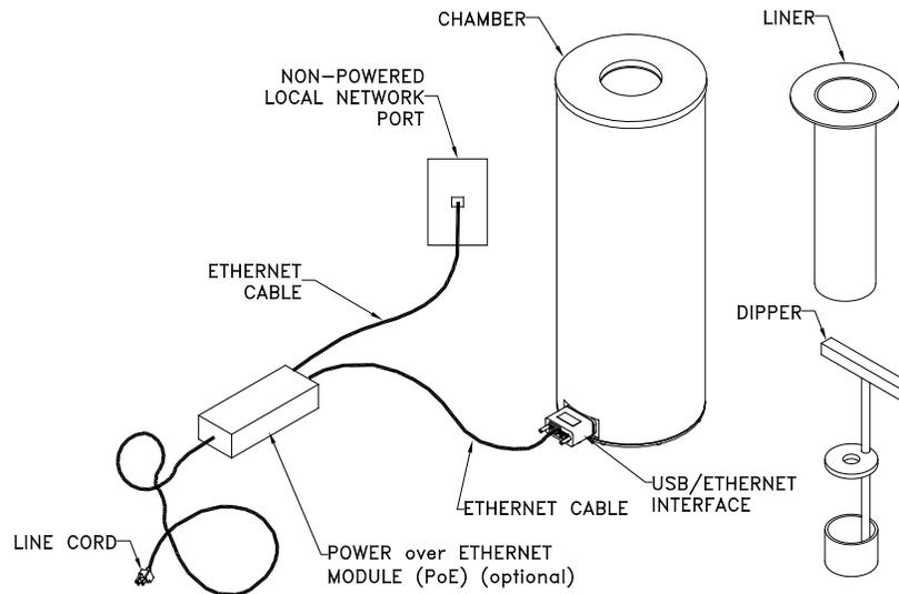
Figure 4-3 Configuration 3 with Optional Accessories
