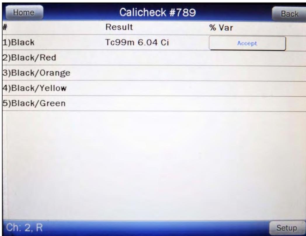
Figure 11-14 Calicheck Linearity Test First Measurement Screen
